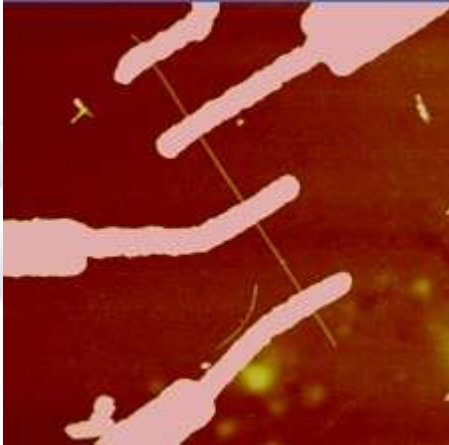
Figure 1: An AFM image of a multiwalled carbon nanotube connected to four microelectrodes.
