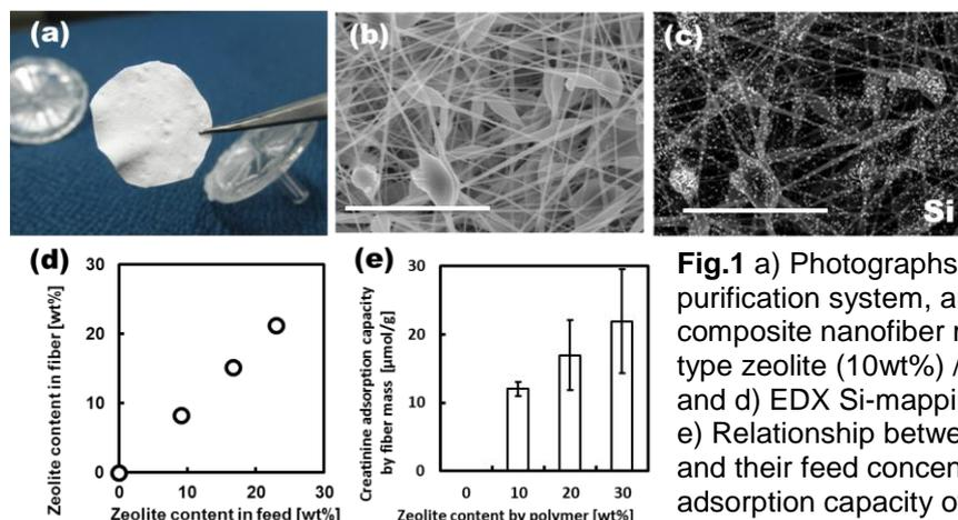
**Fig.1** a) Photographs of a wearable blood purification system, and b) a zeolite-polymer composite nanofiber mesh. c) SEM images of beta-type zeolite (10wt%) / EVOH nanofiber composite, and d) EDX Si-mapping images (scale bar: 8  $\mu\text{m}$ ). e) Relationship between zeolite contents in the fiber and their feed concentrations. f) Creatinine adsorption capacity of beta-type zeolite nanofibers by fiber mass.
