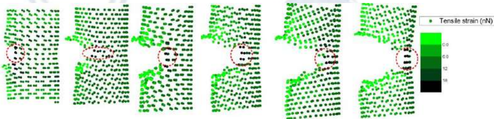
Figure 3 Crack propagation of the vacancy (1C) defect SWMT induced by tensile stress concentration
